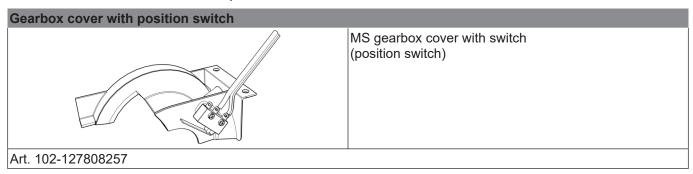
The normal gearbox cover is replaced by the gearbox cover with position switch. The adjustable switch clasp in the gearbox housing actuates the microswitch with floating contact.
