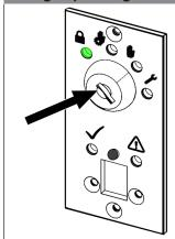
Turn the key switch to the desired operating mode (see chapter operating modes).
