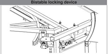
The bistable lock is a bolt lock with two stable end positions (locked, unlocked).
