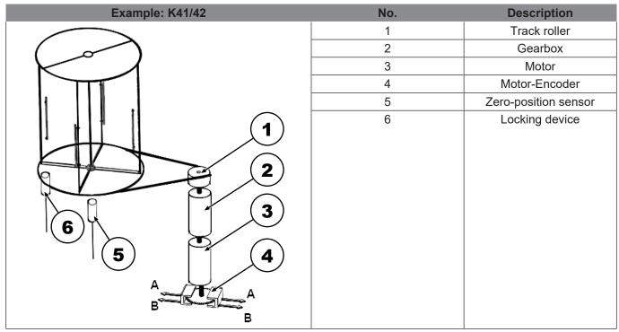
When a user enters the revolving door and presses the turnstile, this is detected by the motor encoder.
